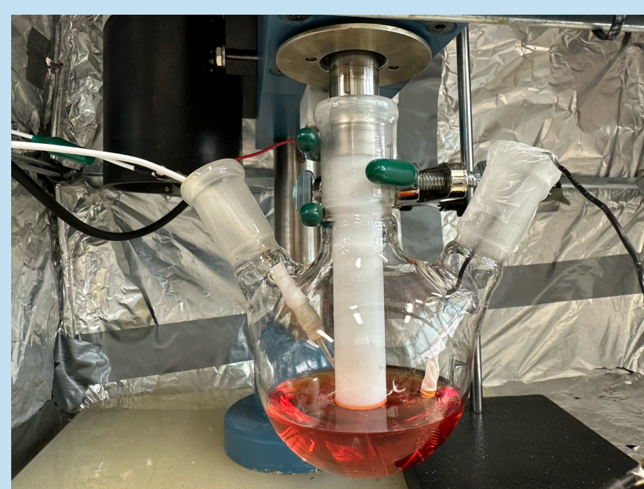
Fig 2. Solution in round bottom flask with electrodes
